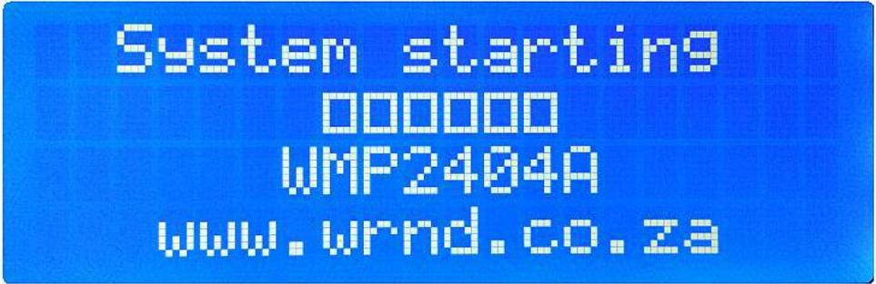
When power is connected to the unit it should briefly display a start-up screen similar to the one above. The model number in this instance is WMP2404A which indicates this unit is a 12/24V, 40A unit. This code will be different for other models according to the following table:
